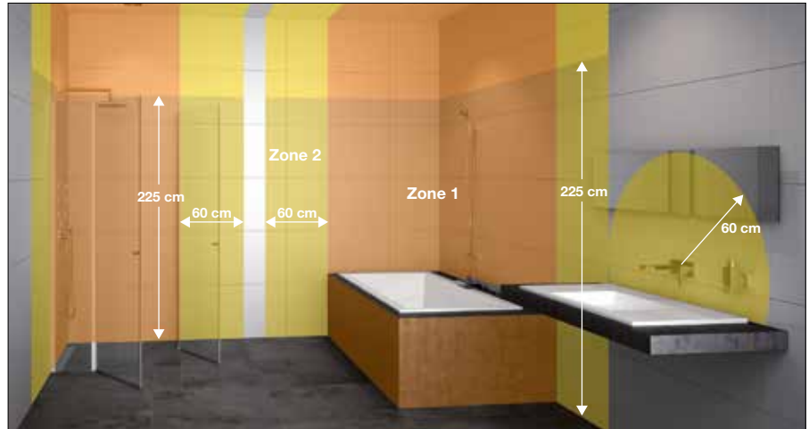
Example: Division of protection zones in bathrooms based on DIN VDE 0100-701
