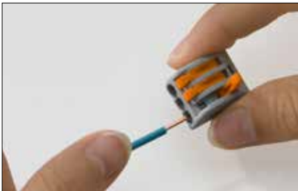
Connect terminal by opening the actuating lever and introducing the conductor
