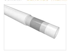
Schlüter-BEKOTEC-THERM-HR is a 5-ply bonded heating pipe made of a high-quality polymer material (PE-RT) with an oxygen diffusion barrier in the centre. The highly flexible heating pipe, which complies with DIN 16833, is optimised for installation in BEKOTEC system panels. Its oxygen tightness is certified according to DIN 4726, and the product is subject to continuous quality monitoring.
