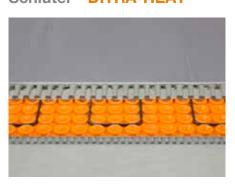
Schlüter-DITRA-HEAT is a polypropylene membrane with a cut back stud structure and an anchoring fleece laminated on the underside. It is a universal substrate for tile coverings, which serves as an uncoupling layer, bonded waterproofing and vapour barrier, designed for the attachment of the matching heating cables for floor and wall heating solution.
