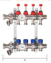
Schlüter-BEKOTEC-THERM-HVT/DE is a heating circuit distributor DN 25 of stainless steel with hot leg and cold leg bars, outside diameter 35 mm.
