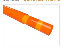
Schlüter-BEKOTEC-THERM-HR is a 5-ply bonded heating pipe made of a high-quality polymer material (PE-RT) with an oxygen diffusion barrier in the centre. The highly flexible heating pipe, which complies with DIN 16833, is optimised for installation in BEKOTEC system panels. Its oxygen tightness is certified according to DIN 4726, and the product is subject to continuous quality monitoring.
