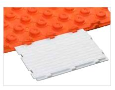
Schlüter-BEKOTEC-ENR is a levelling panel to reduce cutting waste in edge areas and transitions (e.g. doors, niches), for areas in which no heating pipes are installed. It can also be used in front of heating circuit distributors to facilitate heating pipe installation.
