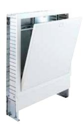
Schlüter-BEKOTEC-THERM-VSE is a distributor cabinet for concealed mounting to house the Schlüter heating circuit distributor manifold and the matching control components. The concealed cabinet consists of fully galvanised steel with perforations in the lateral walls for inserting the connector pipes. The front side (door and frame) is powder coated.
