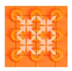
The innovative assembly reduces modular tensions in the screed between the individual studs. The advantage for you: NO control joint profiles in the screed, NO buckling, very short construction times.
