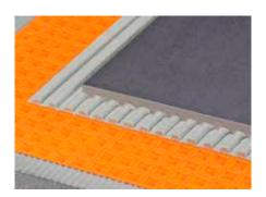
Schlüter-DITRA is a polypropylene membrane with square, dovetailed EasyFill recesses and an anchoring fleece laminated to the underside. In conjunction with tiled coverings, Schlüter-DITRA forms an uncoupling, bonded waterproofing and vapour pressure equalisation layer.
