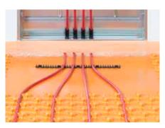
The levelling panel Schlüter-BEKOTEC-ENFGTS is installed in front of heating circuit distributors to simplify the heating pipe installation in the distributor cabinet. The polystyrene panel is adhered to the studded panel with the supplied double sided adhesive tape (6 m). To keep the heating pipe securely within the system, the same impact sound insulation is installed under the levelling panel as with EN 18 FTS.
