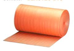
Schlüter-BEKOTEC-BTS is a 5 mm insulation layer of closed cell polyethylene foam for installation below the studded screed panels Schlüter-BEKOTEC-EN-P, -EN-PF and -EN 23 F. The use of BEKOTEC-BTS results in a significant improvement of sound insulation. The material can be used if the required construction height is not sufficient for a thick insulation layer of polystyrene or mineral fibre. The maximum floor load must be limited to 2 kN/m².
