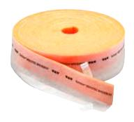
Schlüter-BEKOTEC-BRS/KF is an edge strip of closed cell polyethylene foam with an adhesive leg and an adhesive backing for wall attachment. When the BEKOTEC studded panel is laid on the PE adhesive, the resulting connection prevents flowing screeds from running underneath the assembly during installation.
