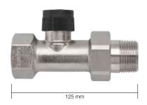
Schlüter-BEKOTEC-THERM-ZV is a heating zone valve that adjusts all heating circuits connected to the heating circuit distributor. The heating zone valve can be controlled by a Schlüter actuator. The operation is controlled via the BEKOTEC control or a DITRA-HEAT-E thermostat. Connection/material: threaded connection/valve 1" (DN 25) of nickel plated brass.
