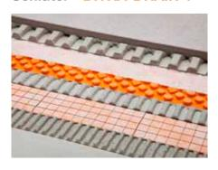
Schlüter-DITRA-DRAIN 4 is an impact resistant polyethylene mat with a special stud structure on one side and a polypropylene webbing laminated on the upper side. It is a universal substrate for tile coverings, which serves as an uncoupling layer and a permanently effective passive capillary drainage mat.
