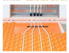
The levelling panel Schlüter-BEKOTEC-ENFGK is installed in front of heating circuit distributors to simplify the heating pipe installation in the distributor cabinet. The polystyrene panel is adhered to the studded panel with the supplied double sided adhesive tape (6 m).
