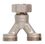
Schlüter-BEKOTEC-THERM-DA is a twin connector made of nickel plated brass that features a 3/4" (DN 20) cone joint nut on one side and two 3/4" (DN 20) cone connector threads on the other side for connecting the Schlüter heating pipes with diameters of 10, 12, 14 or 16 mm.
