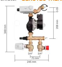
Schlüter-BEKOTEC-THERM-FRS is a fixed-value control station for setting the supply temperature. It enables the installation of a heating circuit distributor (stainless steel or plastic) with 1 to 12 heating circuits. They can be installed in the distributor cabinets VSE/VSV. The fixed-value control supplies the BEKOTEC-THERM ceramic thermal-comfort floor with the required low supply temperatures.
