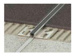
Schlüter-DILEX-KS is a movement profile with edge protection consisting of lateral anchoring legs made of aluminium or stainless steel, which are connected to a replaceable movement zone made of soft synthetic material.
