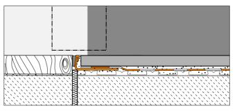
The aim is to build an accessible solution according to DIN as a capillary interruption with a tile covering at the same level (zero threshold).
