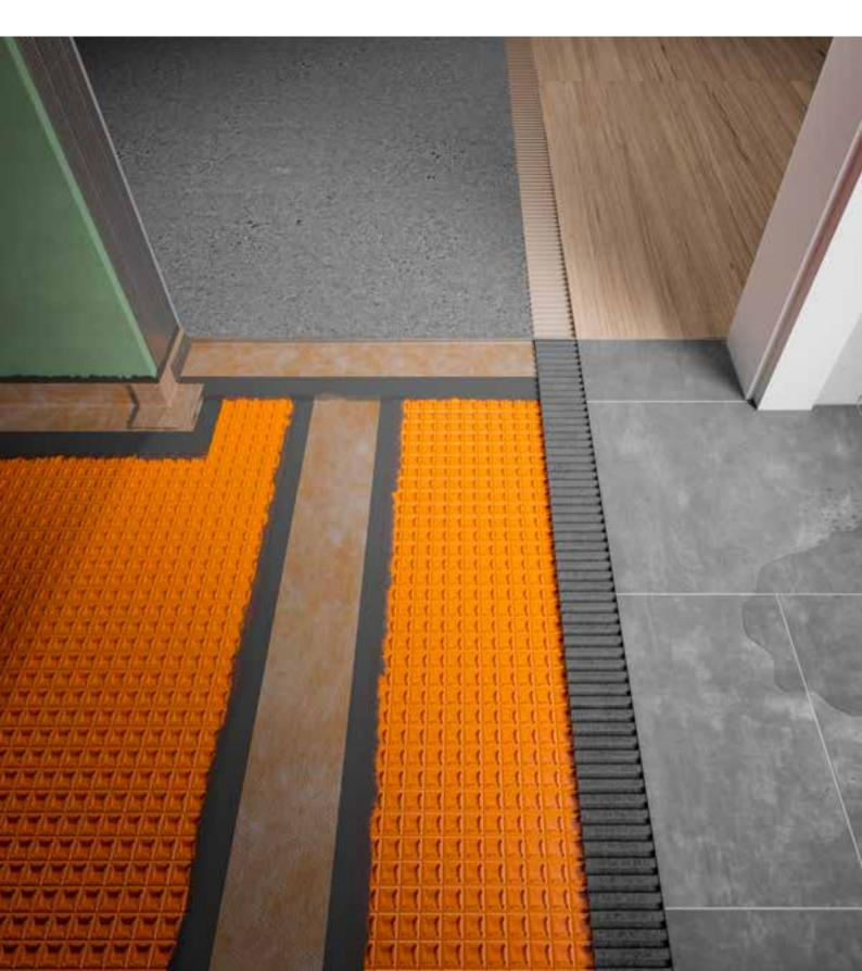
The guidelines for waterproofing interior spaces specify that adjoining rooms without waterproofing must be protected against water exposure from wetrooms, including in door threshold areas. Schlüter-KERDI-CID sets offer the necessary capillary interruption for threshold areas in different door opening configurations.
