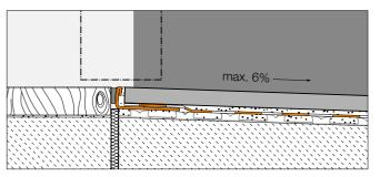
To protect adjoining spaces against any anticipated larger water exposure, tiles may be installed at a slope in the area of the door casing to create a height difference.
