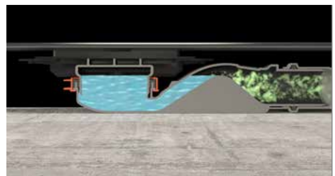
Wave shape creates permanent odour seal
