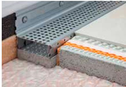
Schlüter-TROBA-LINE-TL is a stainless steel drainage channel that can be installed at low levels to create doorsill or wall connections on balconies and terraces to prevent water accumulation. This can also be used as an area drainage channel.
