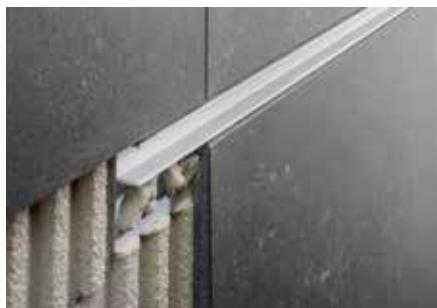
Schlüter-DECO-SG is a decorative profile for joint design in tile coverings. It forms either a 12 mm or 15 mm wide shadow gap. The profile is ideal for holding and fixing glass elements in the floor and wall area.
