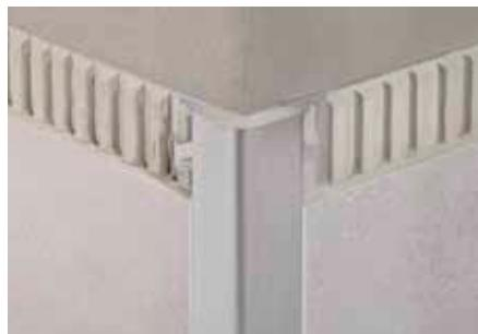
Schlüter-ECK-E is a stainless steel corner profile for external wall corners of tiled surfaces that offers durable edge protection. The perforated anchoring legs are embedded in the tile adhesive during tile installation.
