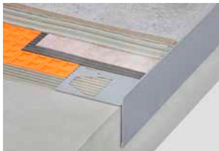
Schlüter-BARA-RT is a T shaped finishing profile of colour coated aluminium for covering exposed edges of balconies and terraces. The top leg covers the edge of the assembly while the lower leg forms a drip edge and hides the joint with the TROBA area drainage mat.
