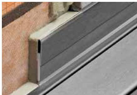
Schlüter-SHOWERPROFILE-R is a two-part wall transition profile for covering the wall area exposed due to the use of a wedge with a linear drainage channel. The profile is available in textured coated or brushed stainless steel. A fleece fabric is laminated on the underside for bonding with the tile adhesive. Due to the two-part design, Schlüter-SHOWERPROFILE-R can be seamlessly adjusted to any height between 23 and 45 mm (available in two versions).
