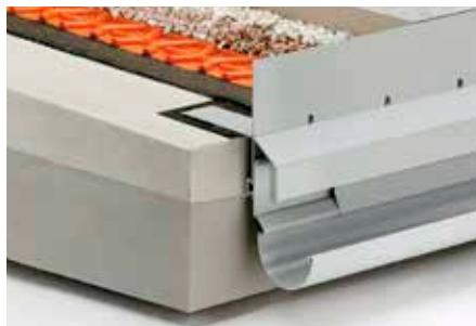
Schlüter-BARA-RKLT is an angled edge profile with drainage holes, made of colour coated aluminium. It is especially suited for large format pavers, which are either installed unbonded over gravel/crushed stone or on pedestals. BARA-RKLT features a T shaped profile chamber for attaching the gutter system Schlüter-BARIN.
