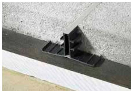
Schlüter-DILEX-EP is a movement joint profile for installation in floating or bonded screeds. The side sections consist of rigid, recycled plastic connected on the top and bottom with soft, grey CPE movement zones.
