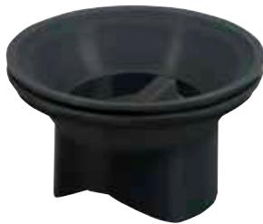
Schlüter-KERDI-DRAIN-R 10 GT is a waterless odour trap for use with all 10 x 10 cm grate and frame sets. It can easily replace the wet trap in our linear drains, being intended for situations when infrequent use of the drain could result in the water in a wet trap evaporating. With a drain capacity of at least 0.4 l/s, it can also permanently replace the standard odour trap unit.
