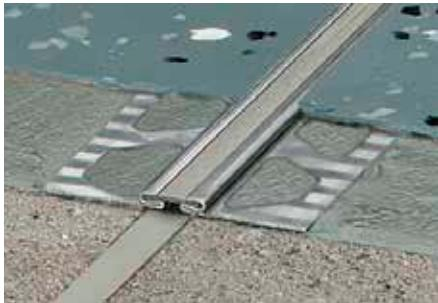
Schlüter-DILEX-EKSB is a movement joint profile with edge protection for floor coatings and other thin floor coverings. It consists of lateral stainless steel anchoring legs that are connected to a fixed elastic insert of soft synthetic material.
