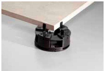
Schlüter-TROBA-LEVEL-PLA 30 are height adapters for supported tile and paver coverings. From an assembly height of 50 mm, one or more TROBA-LEVEL-PLA 30 adapters can be inserted between two Schlüter-TROBA-LEVEL-PL 10 paver supports. TROBA-LEVEL-PLA 30 can be stacked up to a height of 300 mm and can be combined with the paver supports TROBA-LEVEL-PLV 60 and TROBA-LEVEL-LV 3.
