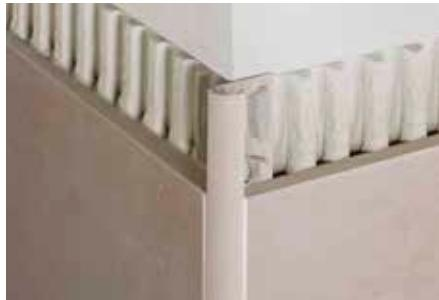
Schlüter®-RONDEC-TS is a symmetrically rounded profile with integrated joint spacer for external wall corners and the edges of tile coverings, made of aluminium with a specially textured coating. The joint spacer creates a uniform grout joint with the tile.
