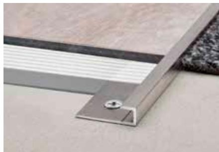
Schlüter-VINPRO-S is an edge profile for resilient coverings (e.g. LVT, vinyl coverings). It is designed to protect the edge of coverings at the transition to other coverings of the same or similar height or at the finishing edge of skirtings.
