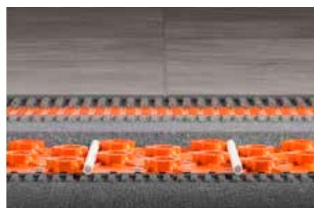
Schlüter-BEKOTEC-EN-FK is a dependable bonded covering assembly system for restoration projects. The system allows for building crack-free, functionally safe screeds and heated screeds in particularly low assembly heights from 20 mm directly on top of load-bearing substrates. In addition to tiles and natural stone, the BEKOTEC screed can also be covered with other flooring materials. (Product data sheet 9.5)
