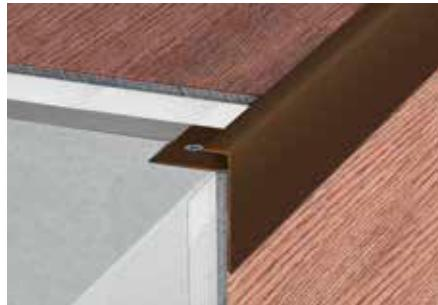
Schlüter-VINPRO-STEP-R is a finishing and edge profile for resilient coverings (e.g. LVT, vinyl coverings) on stairs. The top portion of the profile features a chamfered 10 mm textured footer with rounded front edge, which conceals the cut edge of resilient floor coverings.
