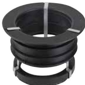
Schlüter-KERDI-DRAIN-ZBS is a conduit gasket for fire protection. It is an alternative to mortar and serves, in conjunction with the vertical floor drain set KD BAV 50 GVB or the vertical stainless steel linear drainage KLV 50 G2, as a fire insulation seal of the core hole drilling ( $\varnothing$  160 mm), while also preventing sound bridges. The product is only approved for fire protection in conjunction with KD BS or KL BS.
