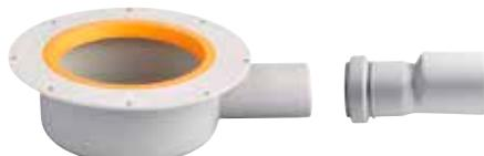
Schlüter-KERDI-DRAIN-BASE is a drain body for combination with the insert KD BV 100 and a grate and frame set with odour trap and gasket seal.
