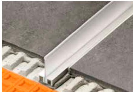
Schlüter-SHOWERPROFILE-WS is a two piece profile of anodised aluminium that serves as a splashguard in floor level showers. The support profile is embedded in the tile adhesive during tile installation. It can be fitted with a semi-circular or upright straight lip to protect against splashing. Both variations are suitable for wheelchair use.
