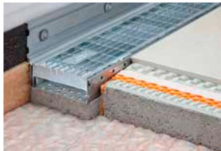
Schlüter-TROBA-LINE-TLR is a drainage channel with a lower part of stainless steel and an upper drainage grate of galvanised steel. It can be installed at low levels to create doorsill or wall connections on balconies and terraces to prevent water accumulation. It can also be used as an area drainage channel for higher water quantities.
