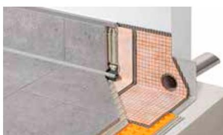
Schlüter-KERDI-DRAIN-SP-E is a stainless steel spout for draining balconies and terraces that are enclosed by a parapet. The supplied Schlüter-KERDI collar is attached to the large adhesive flange for the simple and safe connection to waterproofing assemblies.
