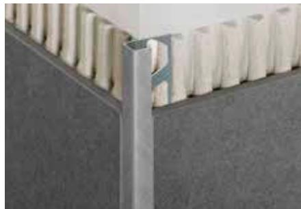
Schlüter-QUADEC-A is a high-quality anodised aluminium finishing profile for external corners and edges of tiled walls. The visible area of the profile forms a right angled external corner. The joint spacer creates a uniform grout joint with the tile.
