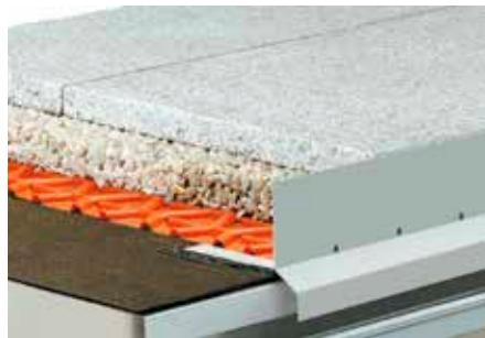
Schlüter-BARA-RKL is an angled edge profile with drainage holes, made of colour coated aluminium. It is especially suited for large format pavers, which are either installed unbonded over gravel/crushed stone or on pedestals.
