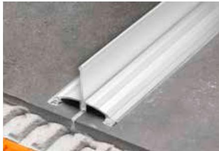
Schlüter-SHOWERPROFILE-WSK is a two-part profile of anodised aluminium that serves as a splashguard in floor-level showers. The support profile is retrofitted to existing coverings. It can be fitted with a semi-circular or upright straight lip to protect against splashing. Both variations are suitable for wheelchair use.
