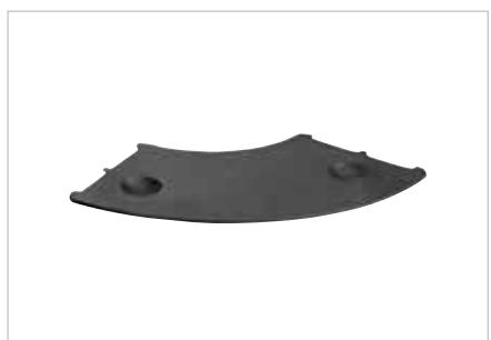
Schlüter-TROBA-LEVEL-AP 1 levelling shims help to adjust the pavers in various slope situations. Differences in tile and paver thickness, uneven areas in the ground or a minor slope can be adjusted by up to 10 mm per corner.
