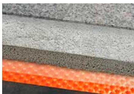
Schlüter-TROBA-PLUS-G is a durable and reliable sub surface drainage system that prevents the possibility of capillary action. The closely positioned conical studs can withstand heavy loads and are covered by a water permeable fleece webbing. The studded mat raises the entire surface assembly, creating a continuous drainage area. Schlüter-TROBA-PLUS 8G is especially suitable for combination with drainage screeds.
