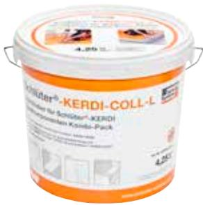
Schlüter-KERDI-COLL-L is a two component sealant adhesive based on a solvent free acrylate dispersion and a reactive cementitious powder. It is suitable for adhering and sealing overlaps of Schlüter-KERDI membranes. In addition, Schlüter-KERDI-COLL-L can be used to tightly adhere the sealing band Schlüter-KERDI-KEBA on bonded waterproofing assemblies made with suitable Schlüter-Systems products as well as on Schlüter-BARA edging profiles.
