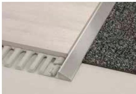
Schlüter-RENO-U is a profile for creating stepless transitions between floor coverings of different heights. The joint spacer creates a uniform grout joint with the tile. Schlüter-RENO-EU, -EBU and -MU do not have a joint spacer.
