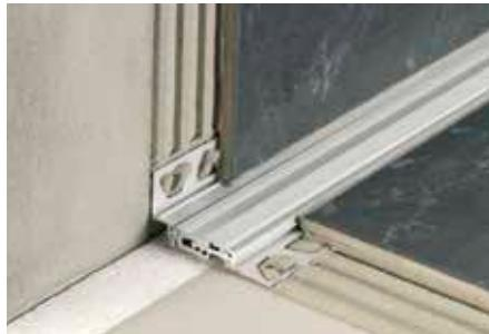
Schlüter-DILEX-BTO is a structural movement profile made of aluminium for floor to wall transitions. The lateral joint connection of the sliding middle section of the profile is able to absorb three dimensional movement.
