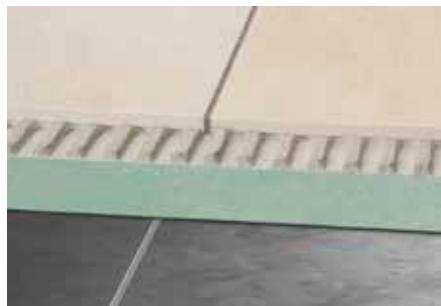
Schlüter-REFLEECE is a fleece mat made of recycled PET with a bonding layer laminated on the underside. It is suitable for creating removable floor coverings made of tiles and natural stone. The self-adhesive underside easily detaches from the substrate during removal without damaging the sub-floor.
