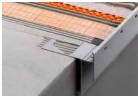
Schlüter-BARA-RAKE is an edge profile with a drip edge for installation over finished sloped screeds. BARA-RAKE is especially suited for assemblies with the bonded drainage mat Schlüter-DITRA-DRAIN. The perforated outer edges give the exterior perimeter of tiled areas a neat appearance.
