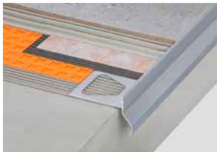
Schlüter-BARA-RKK is a T shaped finishing profile with a short drip edge for installation over finished sloped screeds. It was especially designed for use with the bonded waterproofing membrane Schlüter-DITRA. The closed outer edges give the exterior perimeter of tiled areas a neat appearance.
