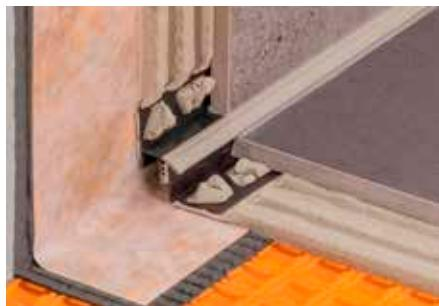
Schlüter-DILEX-EK is a two part profile made of rigid and soft plastic with a tongue and groove connection and an integrated joint chamber for creating durable, flexible and maintenance free perimeter joints between floors and walls or floors and skirtings.
