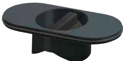
Schlüter-KERDI-LINE-GTO is a waterless odour trap. It can easily replace the wet trap in our linear drains, being intended for situations when infrequent use of the drain could result in the water in a wet trap evaporating. With a drain capacity of at least 0.4 l/s, it can also permanently replace the standard odour trap unit.
