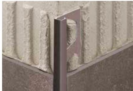
Schlüter-QUADEC-TS is a high-quality finishing profile made of aluminium with a special textured coating for external wall corners and the edges of tile coverings. The visible area of the profile forms a right angled external corner. The joint spacer creates a uniform grout joint with the tile.
