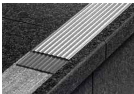
Schlüter-TREP-EFK is a stainless steel stair nosing profile with a special anti-slip tread to create safe and attractive stair treads. It can be adhered with installation adhesive in the corresponding milled grooves or retrofitted on stair steps.
