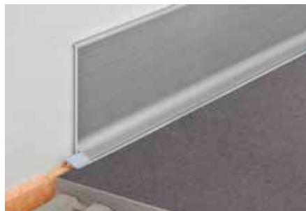
Schlüter-DESIGNBASE-SL-A is a profile made of high-quality coated or anodised aluminium for quickly creating decorative skirtings. The profile is simply attached to the wall area with a suitable adhesive. Optionally, the profile can be equipped with a sealing lip that is available as an accessory to protect the perimeter movement joint from moisture and to reduce the transmission of impact sound.
