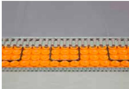
Schlüter-DITRA-HEAT is a polypropylene membrane with a cut back stud structure and an anchoring fleece laminated on the underside. It is a universal substrate for tile coverings, which serves as an uncoupling layer, bonded waterproofing and vapour barrier, designed for the attachment of the matching heating cables for floor and wall heating solution.
