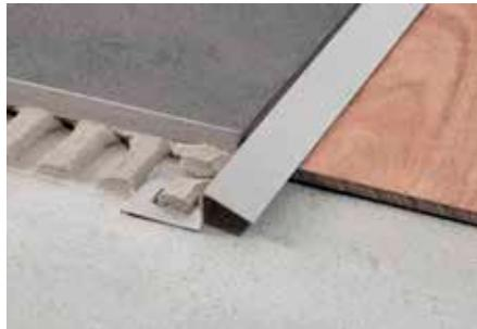
Schlüter-RENO-TK provides a smooth transition between tiled surfaces and adjoining carpeting or other coverings of a lower height. In addition, it effectively protects the edges of the adjacent floor coverings.
