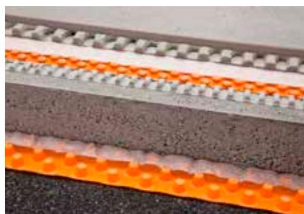
Schlüter-TROBA-PLUS is a durable and reliable sub surface drainage system that prevents the possibility of capillary action. The closely positioned conical studs can withstand heavy loads and are covered by a water permeable fleece webbing. The studded mat raises the entire surface assembly, creating a continuous drainage area.
