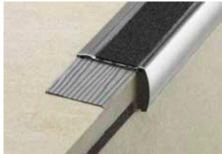
Schlüter-TREP-GK is a stair nosing profile made of brushed stainless steel with an adhered, anti-slip tread. It can be retrofitted to steps with tile or natural stone coverings.
