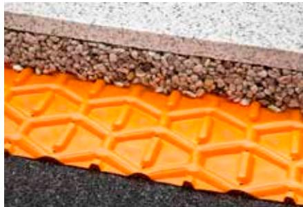
Schlüter-TROBA is a separation and drainage layer for use above a horizontal waterproofing layer and below a screed or gravel layer. It consists of a pressure stable polyethylene sheet with perforated studs for reliable drainage. Tile applications above screeds require the installation of Schlüter-DITRA as an uncoupling and waterproofing membrane. (Product data sheet 7.1)
