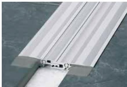
Schlüter-DILEX-BTS is a structural movement profile made of aluminium for retrofitting in finished coverings. The lateral joint connection of the sliding middle section of the profile is able to absorb three dimensional movement.
