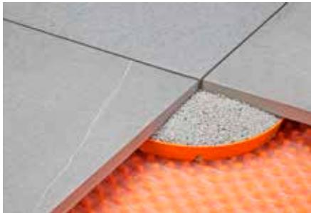
Schlüter-TROBA-STELZ-MR are plastic rings that provide assistance in laying large format pavers on balconies and terraces. The 25 mm high plastic rings are positioned at the cross joints where the pavers meet and are filled with mortar.
