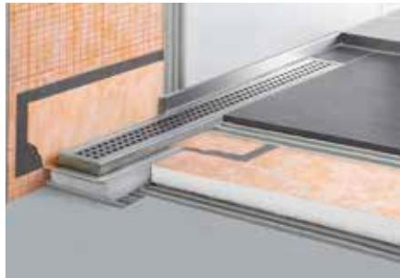
Schlüter-KERDI-LINE-V is a complete set for linear floor-level showers with a vertical drain. It can be positioned at intermediate or perimeter locations in the floor. The perimeter of the channel body consists of an adhesive flange that is coated with a collar made of Schlüter-KERDI. It ensures the reliable connection of the channel body to the bonded waterproofing assembly, both in the floor area and on upright walls.
