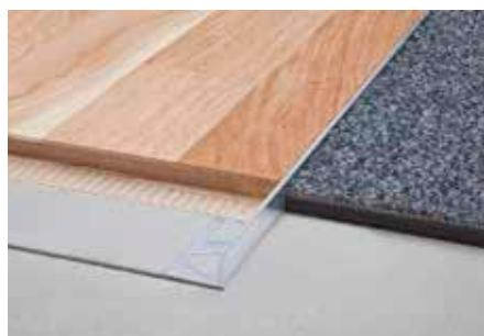
Schlüter-SCHIENE-V is a finishing profile for wooden floors or other rigid covering materials such as terrazzo, with a right angled transition from the anchoring leg to the finishing leg. The evenly shaped finishing leg allows for grinding of the covering.
