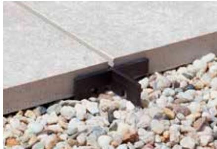
Schlüter-TROBA-ZFK are spacers that ensure an even joint appearance of unbonded assemblies of ceramic, natural stone or concrete pavers in gravel or split stone beds, for example over Schlüter-TROBA. The joint width is 3 mm, the height of the spacers is 15 mm. A height of 30 mm can be achieved by clipping the tile spacers together. (Product data sheet 7.6)
