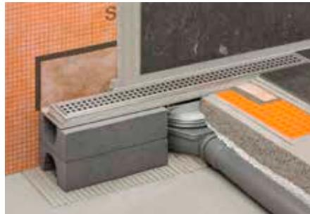
Schlüter-KERDI-LINE-H 50 G2 is a complete set for linear floor-level showers with a horizontal drain. It can be positioned at intermediate or perimeter locations in the floor and features a drain capacity  $\geq 0.8 \text{ l/s}$  according to DIN EN 1253 as well as a water trap height of 50 mm in the odour trap unit. A collar made of Schlüter-KERDI is pre-adhered to the adhesive flange of the channel body for reliable connection to the bonded waterproofing assembly.
