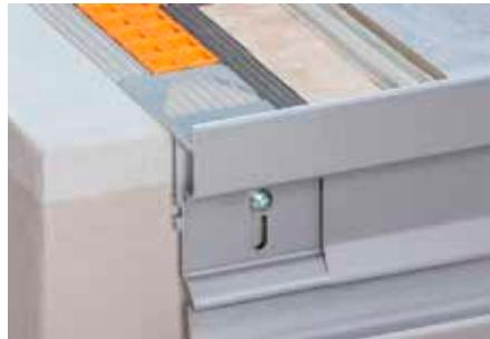
Schlüter-BARA-RTKEG is an edge profile with a drip edge for installation over finished sloped screeds. The profile features a profile chamber for attaching the Schlüter-BARIN gutter system. It is specifically designed for use with the bonded uncoupling membrane Schlüter-DITRA. The closed outer edges give the exterior perimeter of tiled areas a neat appearance.
