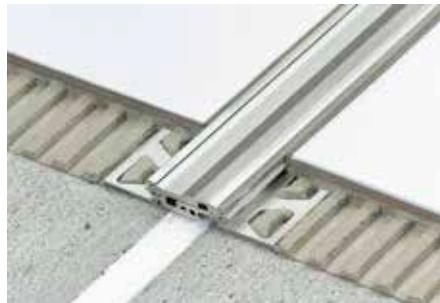
Schlüter-DILEX-BT is a structural expansion joint made of aluminium with lateral joint connections to a sliding telescopic centre section. This allows for absorption of three-dimensional movement.
