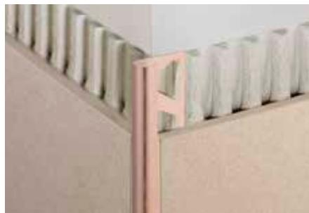
Schlüter-RONDEC-A is a symmetrically rounded profile with an integrated joint spacer for external wall corners or edges of coverings, made of aluminium with different anodised finishes. The joint spacer creates a uniform grout joint with the tile.
