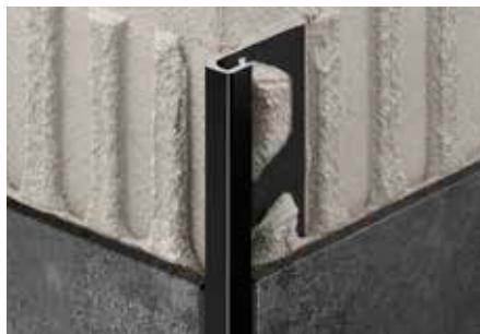
Schlüter-QUADEC-AC is a high-quality colour coated aluminium finishing profile for external corners and the edges of tiled coverings. The visible area of the profile forms a right angled external corner. The joint spacer creates a uniform grout joint with the tile.
