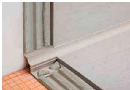
Schlüter-DILEX-AHK-TS is a cove-shaped profile made of aluminium with a special TRENDLINE textured finish. It is suitable for internal wall corners, countertops and shelving with tile and stone coverings. The profile can be combined with Schlüter-RONDEC, -JOLLY, -SCHIENE or -QUADEC profiles in matching textured finishes.
