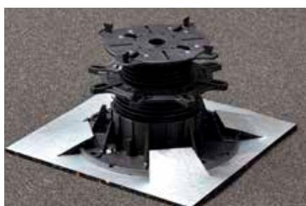
Schlüter-TROBA-LEVEL-PLS 6 are waterproof layer protection pads made of granulated rubber. The paver support bottom of TROBA-LEVEL-PLV 60 or TROBA-LEVEL-LV 3 must be attached in the slit cuts of the protective pads TROBA-LEVEL-PLS 6 (6 mm). In the case of PVC waterproofing assemblies, the aluminium separating layer of the protective pads must be installed face down. If using TROBA-LEVEL-PL 10, these must be placed in the centre of the pads.
