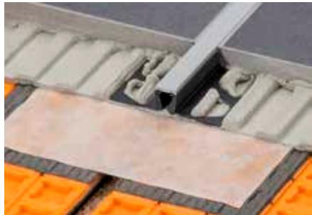
Schlüter-DILEX-BWB is a movement joint profile with lateral sections of rigid, recycled plastic. The top movement zone is made of soft CPE and forms the 10 mm wide visible area.
