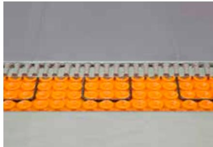
Schlüter-DITRA-HEAT-PS is a polypropylene membrane with a cut back stud structure and a fleece covered in pressure sensitive adhesive laminated to the underside. After peeling off the release film, DITRA-HEAT-PS can be installed on suitable substrates without the use of tile adhesive. Designed to facilitate attachment of the matching heating cables for floor heating it should be used as an uncoupling layer, and a waterproofing and vapour barrier, when installing tiles and other floor coverings.
