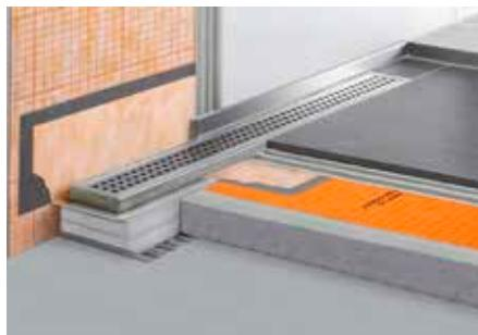
Schlüter-KERDI-LINE-V 50 G2 is a complete set for linear floor-level showers with a vertical drain. It can be positioned at intermediate or perimeter locations in the floor and features a drain capacity  $\geq 0.8 \text{ l/s}$  according to DIN EN 1253 and a water trap height of 50 mm in the odour trap unit. A collar made of Schlüter-KERDI is pre-adhered to the adhesive flange of the channel body for reliable connection to the bonded waterproofing assembly.
