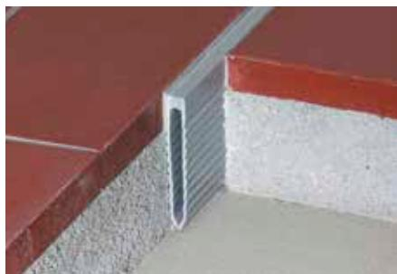
Schlüter-DILEX-MOP is an expansion joint profile with serrated sidewalls made of rigid, recycled PVC and a grey, soft PVC expansion zone for use in screed applications.
