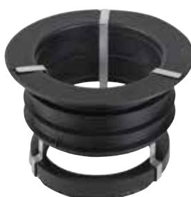
Schlüter-KERDI-DRAIN-ZBS is a conduit gasket for fire protection. It is an alternative to mortar and serves, in conjunction with the vertical floor drain set KD BAV 50 GVB or the vertical stainless steel linear drainage KLV 50 G2, as a fire insulation seal of the core hole drilling (Ø 160 mm), while also preventing sound bridges. The product is only approved for fire protection in conjunction with KD BS or KL BS.
