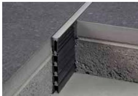
Schlüter-DILEX-EZ 70 is a decorative stress relief profile with undercut sidewalls made of rigid PVC and a soft PVC expansion zone for use in screed installation. The extension segments can be removed to adjust the profile to the height of the assembly.
