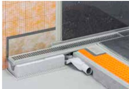
Schlüter-KERDI-LINE-F 40 is a complete set for linear, floor level showers with horizontal drain. It can be positioned at intermediate or perimeter locations in the floor and is particularly well suited for restoration and modernisation projects due to its low assembly height of just 60 mm. A collar made of Schlüter-KERDI is pre-adhered to the adhesive flange of the channel body for reliable connection to the bonded waterproofing assembly.
