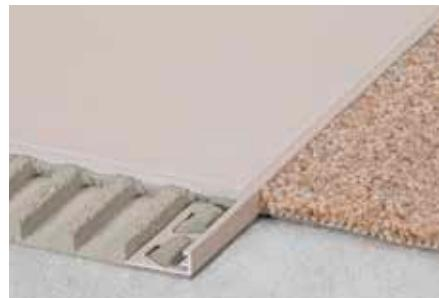
Schlüter-SCHIENE-AC is a decorative profile made of colour coated aluminium. The 87 degree angled finishing leg safeguards tiles against mechanical damage. The joint spacer creates a uniform grout joint with the tile.
