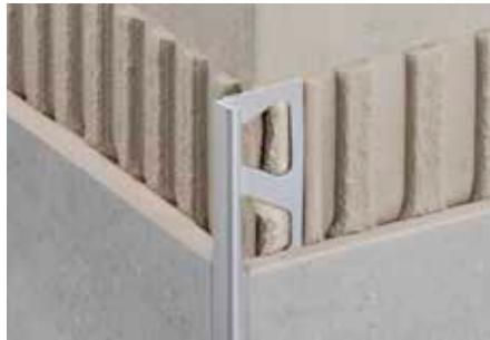
Schlüter-JOLLY is a decorative metal profile to finish and protect tiled external wall corners and other tiled edges, e.g. tiled skirting. The 90 degree angled finishing leg safeguards tiles against mechanical damage. The joint spacers on both sides create a uniform grout joint with the tile. The geometric profile undercutting offers additional bonding surface for the grout. The innovative plug-in connection of the corner pieces results in neat, visually appealing corner connections.
