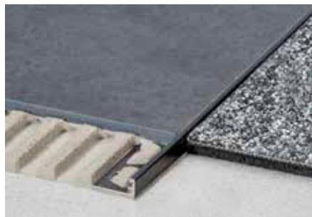
Schlüter-SCHIENE-TS is a decorative profile made of aluminium with a special textured finish that matches modern tile designs. The 87 degree angled finishing leg safeguards tiles against mechanical damage. The joint spacer creates a uniform grout joint with the tile.
