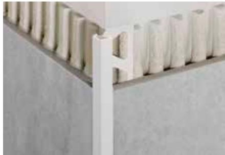
Schlüter-QUADEC-PQ is a finishing profile of coloured PVC for external wall corners and the edges of tile coverings. The visible area of the profile forms a right angled external corner. The joint spacer creates a uniform grout joint with the tile.
