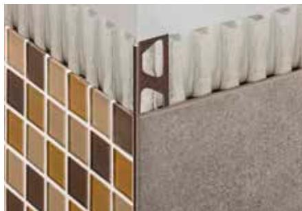
Schlüter-FINEC-TS is a high-quality finishing profile made of anodised aluminium with a special coating structure and texture for the external edges of tile coverings, mosaics or rendered surfaces. The finishing leg of the profile protects the covering edges from mechanical damage and creates an elegant, slim corner detail.
