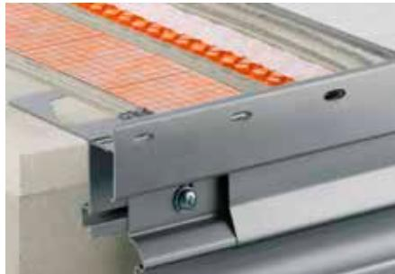
Schlüter-BARA-RTKE is an edge profile with a drip edge for installation over finished sloped screeds. The profile features a profile chamber for attaching the Schlüter-BARIN gutter system. BARA-RTKE is especially suited for assemblies with the bonded drainage mat Schlüter-DITRA-DRAIN. The perforated outer edges give the exterior perimeter of tiled areas a neat appearance.
