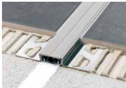
Schlüter-DILEX-KSBT is a structural movement profile with edge protection, consisting of side anchoring legs of aluminium or stainless steel connected to a 20 mm or 30 mm wide movement zone of soft synthetic rubber. (Product data sheet 4.19)
