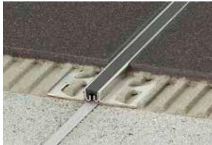
Schlüter-DILEX-KS is a movement profile with edge protection consisting of lateral anchoring legs made of aluminium or stainless steel, which are connected to a replaceable movement zone made of soft synthetic material.
