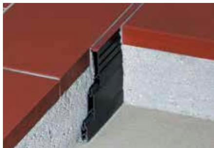
Schlüter-DILEX-MP is an expansion profile with undercut sidewalls made of rigid, recycled PVC and a soft CPE expansion zone covering the sidewalls, complete with extension profiles for use in screed installation.
