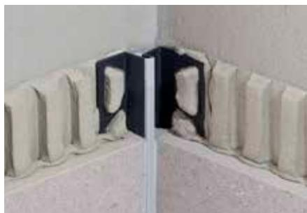
Schlüter-DILEX-EKE is a flexible, single piece corner profile of rigid or soft PVC for internal wall corners or floor-wall transitions. It features an integrated joint chamber and is suitable for use with non-floating covering assemblies.
