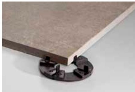
Schlüter-TROBA-LEVEL-PL 10 are stackable supports for tiles and pavers – regardless of their format and thickness. They are made of a special synthetic material with sound insulation effect and can be installed directly over the waterproofing assembly. The 3 mm connectors enable consistent joint appearance and are able to absorb movements in the covering. TROBA-LEVEL-PL 10 can be stacked up to a height of 200 mm and can also be combined with other supports of the product range.
