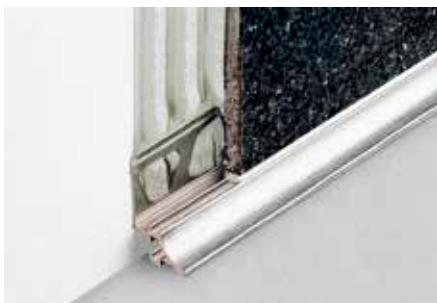
Schlüter-DILEX-AHKA is a cove-shaped aluminium profile for internal wall corners, countertops and shelving with tiled coverings. It is available in a variety of anodised finishes or colour coated aluminium and can be connected to existing coverings on one side.
