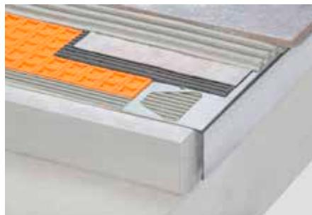
Schlüter-BARA-RW is an angular profile of stainless steel or colour coated aluminium for finishing the exposed perimeters of balconies and terraces.
