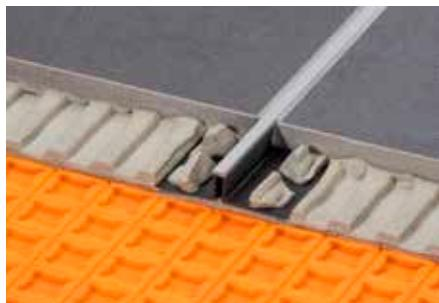
Schlüter-DILEX-BWS is a movement joint profile with lateral sections of rigid, recycled plastic. The movement zone consists of soft CPE and forms the 5 mm wide visible area.
