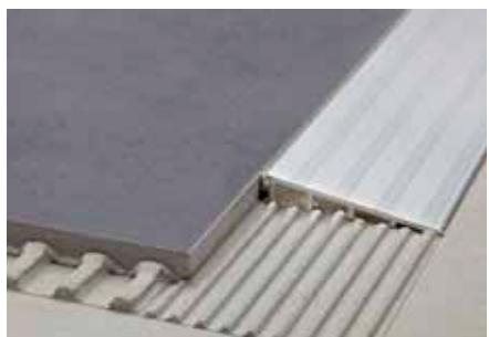
Schlüter-RENO-RAMP-K is a profile for creating stepless transitions between heavily trafficked tile coverings to adjoining coverings of a lower height. The profile can be retrofitted between the covering material and the substrate for subsequent height adjustment.
