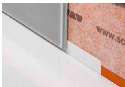
Schlüter-KERDI-CP is a cutting protection that can be shortened to any length and protects the connection seal when the silicone joint is renovated at a later time. The versatile folding profile can be installed directly in the adhesive bed or into freshly applied Schlüter-KERDI-FIX.
