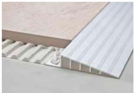
Schlüter-RENO-RAMP is a profile for creating stepless transitions from heavily trafficked tile coverings to adjoining coverings of a lower height. The joint spacer creates a uniform grout joint with the tile.
