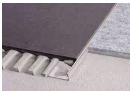
Schlüter-SCHIENE-ES is a stainless steel finishing profile for ceramic tile and natural stone coverings. It features an integrated joint spacer that defines a joint chamber with the covering material.
