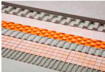
Schlüter-DITRA-DRAIN 4 is an impact resistant polyethylene mat with a special stud structure on one side and a polypropylene webbing laminated on the upper side. It is a universal substrate for tile coverings, which serves as an uncoupling layer and a permanently effective passive capillary drainage mat. (Product data sheet 6.2)
