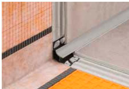
Schlüter-DILEX-HK is a cove-shaped profile of rigid recycled PVC with a cove of soft plastic and an integrated joint chamber for wall to floor joints, which conforms to special hygienic and cleaning requirements such as those of the food processing industry or industrial kitchens.
