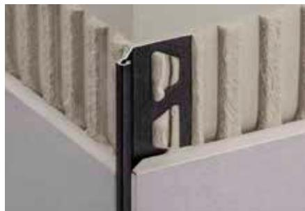
Schlüter-FINEC-SQ is a high-quality finishing profile made of anodised, colour coated or textured aluminium for the external edges of tile coverings. The profile protects the covering edges from mechanical damage and creates an elegant, slim square corner detail.
