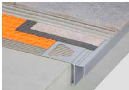
Schlüter-BARA-RAK is a colour coated aluminium balcony edge profile with a drip edge. It is fitted to the edges of finished inclined surfaces to form both an edging and a drip edge. (Product data sheet 5.5)
