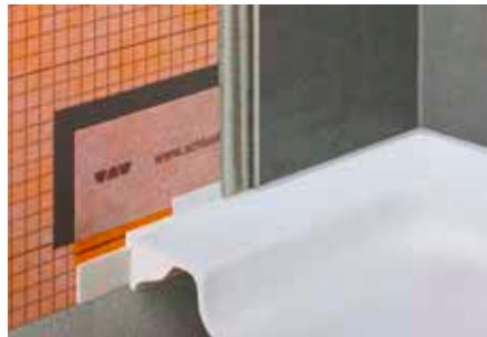
Schlüter-KERDI-TS is a set for creating reliable waterproof connections of building components such as bathtubs and shower trays made of steel enamel, acrylic or mineral casting (according to DIN 18534-1) to the Schlüter-KERDI waterproofing system. It includes a sealing band made of polyethylene with double-sided fleece fabric and self-adhesive sound insulation strip as well as installation materials.
