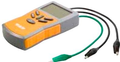
Schlüter-DITRA-HEAT-E-CT is a test device for measuring and checking the resistance of the electrical heating cables Schlüter-DITRA-HEAT-E-HK and the remote sensors supplied with Schlüter-DITRA-HEAT-E thermostats. Designed to monitor the resistance of the heating cables during the entire installation phase, alerting the installer with an audible alarm in the event of damage.
