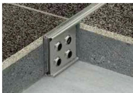
Schlüter-DILEX-EMP is a stainless steel movement joint profile for screeds with a tongue and groove connection to absorb horizontal movements.
