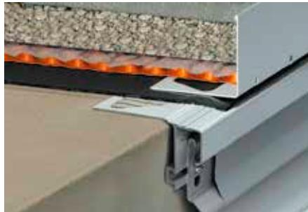
Schlüter-BARA-RWL is an edge profile with drainage holes, made of colour coated aluminium for use on balconies and terraces. It is particularly suitable for finishing coverings on balconies and terraces that are set directly onto a gravel layer or pedestals.
