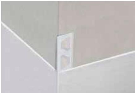
Schlüter-FINEC-A is a high-quality finishing profile made of anodised or colour coated aluminium for the external edges of tile coverings, mosaics or rendered surfaces. The finishing leg of the profile protects the covering edges from mechanical damage and creates an elegant, slim corner detail.
