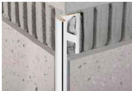
Schlüter-DECO is a profile with a 6 mm wide visible surface for decorative joint design in tile coverings. Schlüter-DECO-M and -MC can also be used as finishing profiles for external wall corners. Schlüter-DECO of aluminium, brass and stainless steel is also suitable for designing floor coverings.
