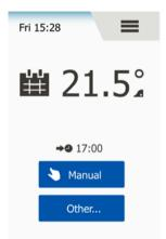
The thermostat allows you to control temperature automatically according to a weekly schedule of your choice. The thermostat comes with a pre-programmed schedule for easy and economic heating control of most homes, see Factory Settings: Preset Schedule.
